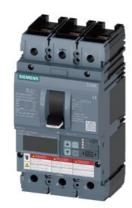
Circuit breaker 3VA6 UL Frame 150 breaking capacity class C 100kA @ 480 V 3pole, Line protection ETU856, LSI, In=150A overload protection, 100% rated Ir=60A ...150A Short-circuit protection Isd=0.6..10x In, Ii=1.5..10x In N conductor protection optionally with external CT; up to 160% Ground-fault alarm message via EFB300 or COM nut keeper kit on both sides
