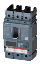
Circuit breaker 3VA6 UL Frame 150 breaking capacity class C 100kA @ 480V 3-pole, Line protection ETU856, LSI, In=150A overload protection, 100% rated Ir=60A...150A Short-circuit protection Isd=0.6..10x In, Ii=1.5..10x In N conductor protection optionally with external CT, up to 160% Ground-fault alarm message via EFB300 or COM without connection
