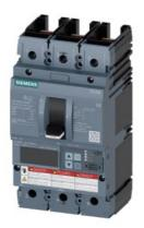
circuit breaker 3VA6 UL frame 150 breaking capacity class C 100kA @ 480V 3-pole, line protection ETU856, LSI, In=150A overload protection Ir=60A...150A short-circuit protection Isd=0.6..10x In, Ii=1.5..10x In N conductor protection optionally with external current transformer, up to 160% ground-fault alarm message via EFB300 or COM without connection
