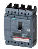
Circuit breaker 3VA6 UL Frame 150 breaking capacity class C 100kA @ 480V 4-pole, Line protection ETU860, LSIG, In=150A overload protection, 100% rated Ir=60A...150A Short-circuit protection Isd=0.6..10x In, Ii=1.5..10x In N conductor protection adjustable (OFF, up to 100%) Ground-fault protection Ig=0.2...1 x In= tg=0.05-0.8s without connection
