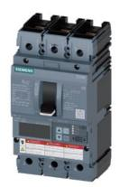
Circuit breaker 3VA6 UL Frame 150 breaking capacity class C 100kA @ 480 V 3-pole, Line protection ETU860, LSIG, In=150A overload protection, 100% rated Ir=60A ...150A Short-circuit protection Isd=0.6..10x In, Ii=1.5..10x In N conductor protection optionally with external CT; up to 160% Ground-fault protection Ig=0.2... 1 x In, tg=0.05-0.8s nut keeper kit on both sides
