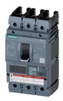
Circuit breaker 3VA6 UL Frame 150 breaking capacity class C 100kA @ 480V 3-pole, Line protection ETU850, LSI, In=150A overload protection, 100% rated Ir=60A...150A Short-circuit protection Isd=0.6..10x In, Ii=1.5..10x In N conductor protection optionally with external CT, up to 160% without connection
