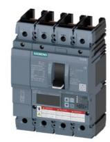
Circuit breaker 3VA6 UL Frame 150 breaking capacity class C 100kA @ 480V 4pole, Line protection ETU830, LIG, In=150A overload protection, 100% rated Ir=60A...150A Short-circuit protection Ii=1.5...10 x In Ground-fault protection Ig=0.2...1 x In, tg=0.05-0.8s without connection
