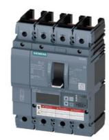
circuit breaker 3VA6 UL frame 150 breaking capacity class C 100kA @ 480V 4-pole, line protection ETU830, LIG, In=150A overload protection Ir=60A...150A short-circuit protection Ii=1.5...10 x In ground-fault protection Ig=0.2...1 x In, tg=0.05-0.8s without connection
