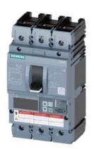
Circuit breaker 3VA6 UL Frame 150 breaking capacity class C 100kA @ 480 V 3-pole, Line protection ETU830, LIG, In=150A overload protection, 100% rated Ir=60A ...150A Short-circuit protection Ii=1.5...10 x In Ground-fault protection Ig=0.2... 1 x In, tg=0.05-0.8s cable connection on both sides
