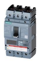
circuit breaker 3VA6 UL frame 150 breaking capacity class C 100kA @ 480 V 3-pole, line protection ETU830, LIG, In=150A overload protection Ir=60A ...150A short-circuit protection Ii=1.5...10 x In ground-fault protection Ig=0.2... 1 x In, tg=0.05-0.8s cable connection on both sides
