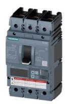
Circuit breaker 3VA6 UL Frame 150 breaking capacity class C 100kA @ 480 V 3-pole, Line protection ETU830, LIG, In=150A overload protection, 100% rated Ir=60A ...150A Short-circuit protection Ii=1.5...10 x In Ground-fault protection Ig=0.2... 1 x In, tg=0.05-0.8s nut keeper kit on both sides
