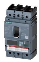
circuit breaker 3VA6 UL frame 150 breaking capacity class C 100kA @ 480 V 3-pole, line protection ETU830, LIG, In=150A overload protection Ir=60A ...150A short-circuit protection li=1.5...10 x ln ground-fault protection Ig=0.2... 1 x In, tg=0.05-0.8s nut keeper kit on both sides
