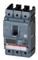
circuit breaker 3VA6 UL frame 150 breaking capacity class C 100kA @ 480V 3-pole, line protection ETU830, LIG, ln=150A overload protection lr=60A...150A short-circuit protection li=1.5...10 x ln ground-fault protection lg=0.2...1 x ln, tg=0.05-0.8s without connection
