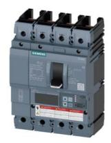
Circuit breaker 3VA6 UL Frame 150 breaking capacity class C 100kA @ 480V 4-pole, Line protection ETU820, LI, In=150A overload protection, 100% rated Ir=60A...150A Short-circuit protection Ii=1.5...10 x In without connection
