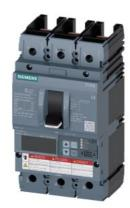
Circuit breaker 3VA6 UL Frame 150 breaking capacity class C 100kA @ 480V 3-pole, Line protection ETU820, LI, In=150A overload protection, 100% rated Ir=60A...150A Short-circuit protection Ii=1.5...10 x In without connection
