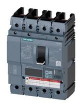
Circuit breaker 3VA6 UL Frame 150 breaking capacity class C 100kA @ 480V 4-pole, Line protection ETU556, LSI, In=150A overload protection, 100% rated Ir=60A...150A Short-circuit protection Isd=0.6..10x In, Ii=1.5..10x In N conductor protection adjustable (OFF, up to 100%) Ground-fault alarm message via EFB300 or COM without connection
