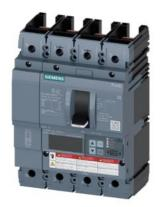
circuit breaker 3VA6 UL frame 150 breaking capacity class C 100kA @ 480V 4-pole, line protection ETU556, LSI, In=150A overload protection Ir=60A...150A short-circuit protection Isd=0.6..10x In, Ii=1.5..10x In N conductor protection adjustable (OFF, up to 100%) ground-fault alarm message via EFB300 or COM without connection
