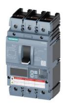
Circuit breaker 3VA6 UL Frame 150 breaking capacity class C 100kA @ 480 V 3-pole, Line protection ETU556, LSI, In=150A overload protection, 100% rated Ir=60A ...150A Short-circuit protection Isd=0.6..10x In, Ii=1.5..10x In N conductor protection optionally with external CT; up to 160% Ground-fault alarm message via EFB300 or COM cable connection on both sides
