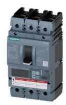
Circuit breaker 3VA6 UL Frame 150 breaking capacity class C 100kA @ 480 V 3pole, Line protection ETU556, LSI, In=150A overload protection, 100% rated Ir=60A ...150A Short-circuit protection Isd=0.6..10x In, Ii=1.5..10x In N conductor protection optionally with external CT; up to 160% Ground-fault alarm message via EFB300 or COM nut keeper kit on both sides
