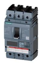
circuit breaker 3VA6 UL frame 150 breaking capacity class C 100kA @ 480 V 3-pole, line protection ETU556, LSI, In=150A overload protection Ir=60A ...150A short-circuit protection Isd=0.6..10x In, Ii=1.5..10x In N conductor protection opt. w. ext. CT; up to 160% ground-fault alarm message via EFB300 or COM nut keeper kit on both sides
