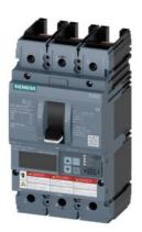
circuit breaker 3VA6 UL frame 150 breaking capacity class C 100kA @ 480V 3-pole, line protection ETU556, LSI, In=150A overload protection Ir=60A...150A short-circuit protection Isd=0.6..10x In, Ii=1.5..10x In N conductor protection optionally with external current transformer, up to 160% ground-fault alarm message via EFB300 or COM without connection
