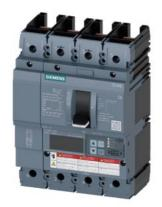
Circuit breaker 3VA6 UL Frame 150 breaking capacity class C 100kA @ 480V 4-pole, Line protection ETU560, LSIG, In=150A overload protection, 100% rated Ir=60A...150A Short-circuit protection Isd=0.6..10x In, Ii=1.5..10x In N conductor protection adjustable (OFF, up to 100%) Ground-fault protection Ig=0.2...1 x In=tg=0.05-0.8s without connection
