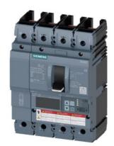
circuit breaker 3VA6 UL frame 150 breaking capacity class C 100kA @ 480V 4-pole, line protection ETU560, LSIG, In=150A overload protection Ir=60A...150A short-circuit protection Isd=0.6..10x In, Ii=1.5..10x In N conductor protection adjustable (OFF, up to 100%) ground-fault protection Ig=0.2...1 x In= tg=0.05-0.8s without connection
