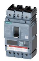
Circuit breaker 3VA6 UL Frame 150 breaking capacity class C 100kA @ 480 V 3pole, Line protection ETU560, LSIG, In=150A overload protection, 100% rated Ir=60A ...150A Short-circuit protection Isd=0.6..10x In, Ii=1.5..10x In N conductor protection optionally with external CT; up to 160% Ground-fault protection Ig=0.2... 1 x In, tg=0.05-0.8s cable connection on both sides
