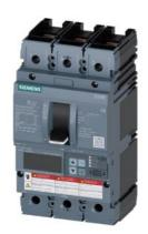
Circuit breaker 3VA6 UL Frame 150 breaking capacity class C 100kA @ 480 V 3-pole, Line protection ETU560, LSIG, In=150A overload protection, 100% rated Ir=60A ...150A Short-circuit protection Isd=0.6..10x In, Ii=1.5..10x In N conductor protection optionally with external CT; up to 160% Ground-fault protection Ig=0.2... 1 x In, tg=0.05-0.8s nut keeper kit on both sides
