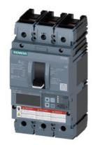
circuit breaker 3VA6 UL frame 150 breaking capacity class C 100kA @ 480 V 3-pole, line protection ETU560, LSIG, In=150A overload protection Ir=60A ...150A short-circuit protection Isd=0.6..10x In, Ii=1.5..10x In N conductor protection opt. w. ext. CT; up to 160% ground-fault protection Ig=0.2... 1 x In, tg=0.05-0.8s nut keeper kit on both sides
