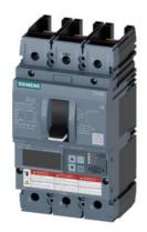
Circuit breaker 3VA6 UL Frame 150 breaking capacity class C 100kA @ 480V 3-pole, Line protection ETU560, LSIG, In=150A overload protection, 100% rated Ir=60A...150A Short-circuit protection Isd=0.6..10x In, Ii=1.5..10x In N conductor protection optionally with external CT, up to 160% Ground-fault protection Ig=0.2...1 x In, tg=0.05-0.8s without connection
