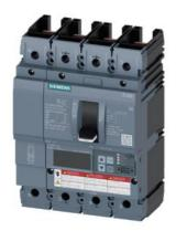
Circuit breaker 3VA6 UL Frame 150 breaking capacity class C 100kA @ 480V 4-pole, Line protection ETU550, LSI, ln=150A overload protection, 100% rated lr=60A...150A Short-circuit protection lsd=0.6..10x In, li=1.5..10x In N conductor protection adjustable (OFF, up to 100%) without connection
