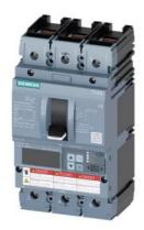
Circuit breaker 3VA6 UL Frame 150 breaking capacity class C 100kA @ 480 V 3-pole, Line protection ETU550, LSI, In=150A overload protection, 100% rated Ir=60A ...150A Short-circuit protection Isd=0.6..10x In, Ii=1.5..10x In N conductor protection optionally with external CT; up to 160% cable connection on both sides
