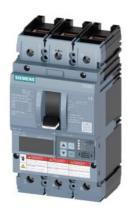
circuit breaker 3VA6 UL frame 150 breaking capacity class C 100kA @ 480 V 3-pole, line protection ETU550, LSI, In=150A overload protection Ir=60A ...150A short-circuit protection Isd=0.6..10x In, Ii=1.5..10x In N conductor protection opt. w. ext. CT; up to 160% cable connection on both sides
