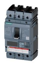
Circuit breaker 3VA6 UL Frame 150 breaking capacity class C 100kA @ 480 V 3pole, Line protection ETU550, LSI, In=150A overload protection, 100% rated Ir=60A ...150A Short-circuit protection Isd=0.6..10x In, Ii=1.5..10x In N conductor protection optionally with external CT; up to 160% nut keeper kit on both sides
