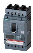
circuit breaker 3VA6 UL frame 150 breaking capacity class C 100kA @ 480 V 3-pole, line protection ETU550, LSI, In=150A overload protection Ir=60A ...150A short-circuit protection Isd=0.6..10x In, Ii=1.5..10x In N conductor protection opt. w. ext. CT; up to 160% nut keeper kit on both sides
