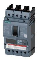
Circuit breaker 3VA6 UL Frame 150 breaking capacity class C 100kA @ 480V 3-pole, Line protection ETU550, LSI, In=150A overload protection, 100% rated Ir=60A...150A Short-circuit protection Isd=0.6..10x In, Ii=1.5..10x In N conductor protection optionally with external CT, up to 160% without connection
