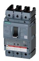
Circuit breaker 3VA6 UL Frame 150 breaking capacity class C 100kA @ 480V 3-pole, Line protection ETU350, LSI, In=150A overload protection, 100% rated Ir=60A...150A Short-circuit protection Isd=1.5...10 x Ir, Ii=10 x In without connection
