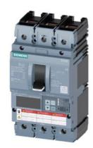
circuit breaker 3VA6 UL frame 150 breaking capacity class H 65kA @ 480 V 3pole, line protection ETU856, LSI, In=150A overload protection Ir=60A ...150A short-circuit protection Isd=0.6..10x In, Ii=1.5..10x In N conductor protection opt. w. ext. CT; up to 160% ground-fault alarm message via EFB300 or COM cable connection on both sides
