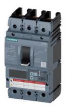
Circuit breaker 3VA6 UL Frame 150 breaking capacity class H 65kA @ 480V 3-pole, Line protection ETU856, LSI, In=150A overload protection, 100% rated Ir=60A...150A Short-circuit protection Isd=0.6..10x In, Ii=1.5..10x In N conductor protection optionally with external CT, up to 160% Ground-fault alarm message via EFB300 or COM without connection
