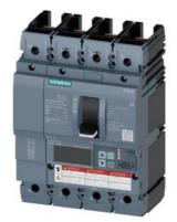
circuit breaker 3VA6 UL frame 150 breaking capacity class H 65kA @ 480V 4-pole, line protection ETU830, LIG, In=150A overload protection Ir=60A...150A short-circuit protection Ii=1.5...10 x In ground-fault protection Ig=0.2...1 x In, tg=0.05-0.8s without connection
