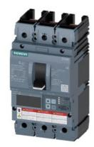
Circuit breaker 3VA6 UL Frame 150 breaking capacity class H 65kA @ 480V 3-pole, Line protection ETU830, LIG, In=150A overload protection, 100% rated Ir=60A...150A Short-circuit protection Ii=1.5...10 x In Ground-fault protection Ig=0.2...1 x In, tg=0.05-0.8s without connection
