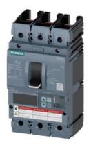
circuit breaker 3VA6 UL frame 150 breaking capacity class H 65kA @ 480V 3-pole, line protection ETU830, LIG, In=150A overload protection Ir=60A...150A short-circuit protection Ii=1.5...10 x In ground-fault protection Ig=0.2...1 x In, tg=0.05-0.8s without connection
