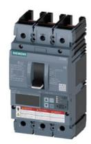
Circuit breaker 3VA6 UL Frame 150 breaking capacity class H 65kA @ 480V 3-pole, Line protection ETU550, LSI, In=150A overload protection, 100% rated Ir=60A...150A Short-circuit protection Isd=0.6..10x In, Ii=1.5..10x In N conductor protection optionally with external CT, up to 160% without connection
