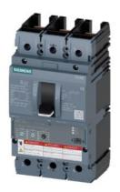
Circuit breaker 3VA6 UL Frame 150 breaking capacity class H 65kA @ 480V 3-pole, Line protection ETU320, LI, In=150A overload protection, 100% rated Ir=60A...150A Short-circuit protection Ii=1.5...10 x In without connection
