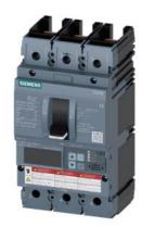
Circuit breaker 3VA6 UL Frame 150 breaking capacity class M 35kA @ 480V 3pole, Line protection ETU856, LSI, In=150A overload protection, 100% rated Ir=60A...150A Short-circuit protection Isd=0.6..10x In, Ii=1.5..10x In N conductor protection optionally with external CT, up to 160% Ground-fault alarm message via EFB300 or COM without connection
