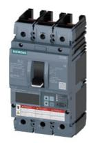
circuit breaker 3VA6 UL frame 150 breaking capacity class M 35kA @ 480V 3pole, line protection ETU856, LSI, In=150A overload protection Ir=60A...150A short-circuit protection Isd=0.6..10x In, Ii=1.5..10x In N conductor protection optionally with external current transformer, up to 160% ground-fault alarm message via EFB300 or COM without connection
