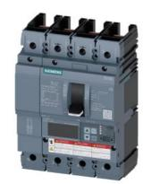
Circuit breaker 3VA6 UL Frame 150 breaking capacity class M 35kA @ 480V 4pole, Line protection ETU850, LSI, In=150A overload protection, 100% rated Ir=60A...150A Short-circuit protection Isd=0.6..10x In, Ii=1.5..10x In N conductor protection adjustable (OFF, up to 100%) without connection
