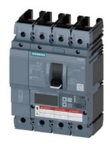
circuit breaker 3VA6 UL frame 150 breaking capacity class M 35kA @ 480V 4-pole, line protection ETU830, LIG, In=150A overload protection Ir=60A...150A short-circuit protection Ii=1.5...10 x In ground-fault protection Ig=0.2...1 x In, tg=0.05-0.8s without connection
