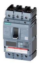
Circuit breaker 3VA6 UL Frame 150 breaking capacity class M 35kA @ 480 V 3-pole, Line protection ETU830, LIG, In=150A overload protection, 100% rated Ir=60A ...150A Short-circuit protection Ii=1.5...10 x In Ground-fault protection Ig=0.2... 1 x In, tg=0.05-0.8s cable connection on both sides
