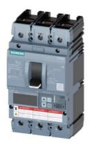
circuit breaker 3VA6 UL frame 150 breaking capacity class M 35kA @ 480 V 3-pole, line protection ETU830, LIG, ln=150A overload protection Ir=60A ...150A short-circuit protection li=1.5...10 x ln ground-fault protection lg=0.2... 1 x ln, tg=0.05-0.8s cable connection on both sides
