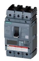
Circuit breaker 3VA6 UL Frame 150 breaking capacity class M 35kA @ 480 V 3pole, Line protection ETU830, LIG, In=150A overload protection, 100% rated Ir=60A ...150A Short-circuit protection li=1.5...10 x In Ground-fault protection Ig=0.2... 1 x In, tg=0.05-0.8s nut keeper kit on both sides
