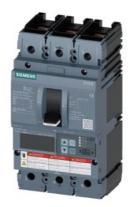
circuit breaker 3VA6 UL frame 150 breaking capacity class M 35kA @ 480 V 3-pole, line protection ETU830, LIG, ln=150A overload protection Ir=60A ...150A short-circuit protection li=1.5...10 x ln ground-fault protection lg=0.2... 1 x ln, tg=0.05-0.8s nut keeper kit on both sides
