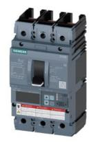
Circuit breaker 3VA6 UL Frame 150 breaking capacity class M 35kA @ 480V 3-pole, Line protection ETU830, LIG, In=150A overload protection, 100% rated Ir=60A...150A Short-circuit protection Ii=1.5...10 x In Ground-fault protection Ig=0.2...1 x In, tg=0.05-0.8s without connection
